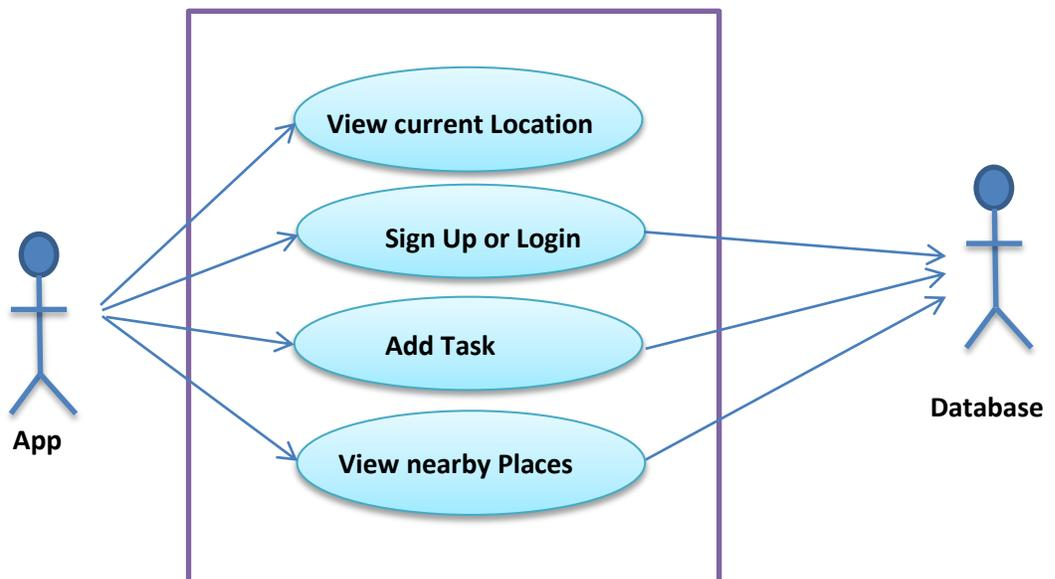
Fig: Use Case Diagram of the application
